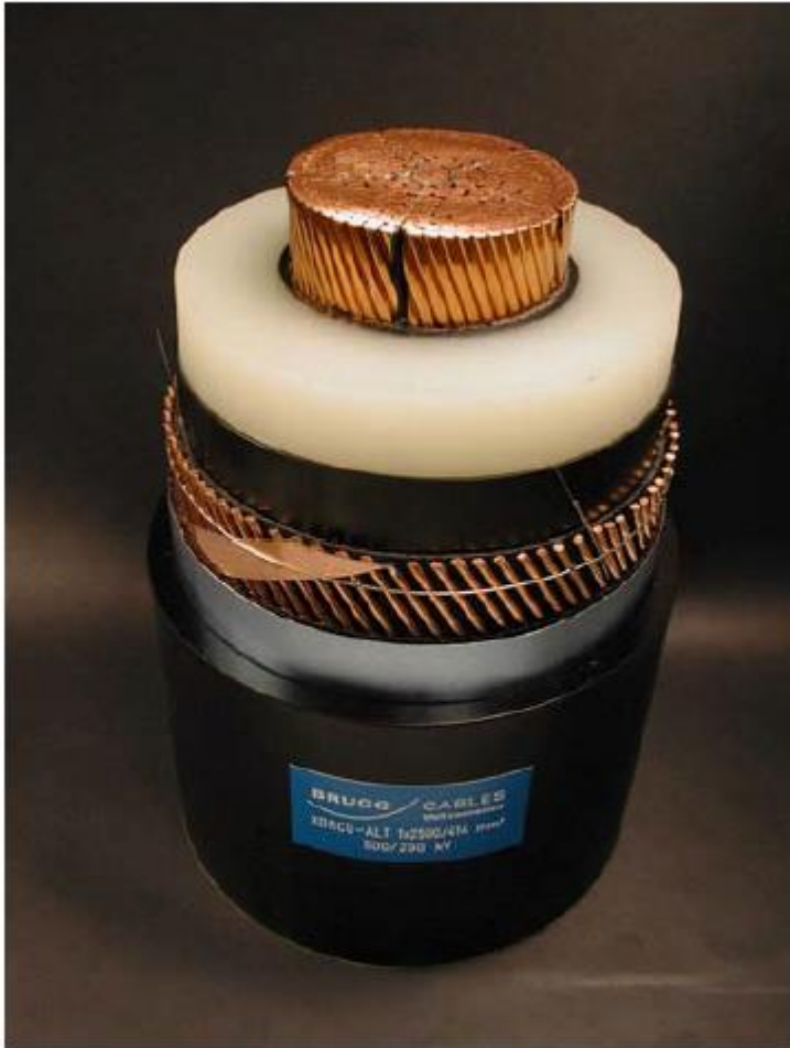
Typical sample of a 2500mm 2 500 kV XLPE cable
